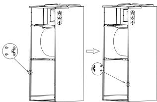
8. Reinstall the evaporator and drain pan.
