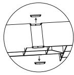
Remove knockouts as shown in the figure.
