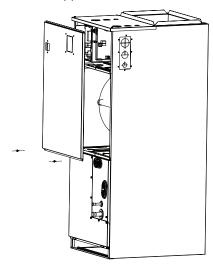
14. Reinstal the flter and flter cover plate.
