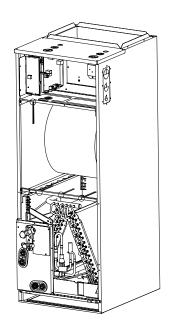
6. Take out the evaporator and drain pan and rotate 180°.
